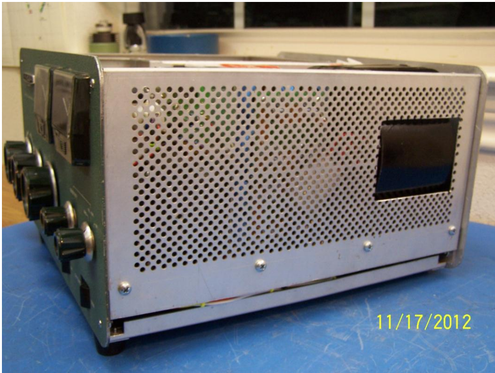
Photo 13 - It was necessary to cut a rectangular hole in the right-side panel to make room for the Harbach transformer. The transformer will not interfere with the outer enclosure for the amp.
